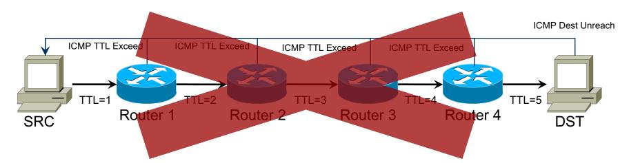
All returned ICMP packets must travel to the end of the LSP before going back to the sender. This makes every hop in the LSP appear to have the same RTT as the final hop.
