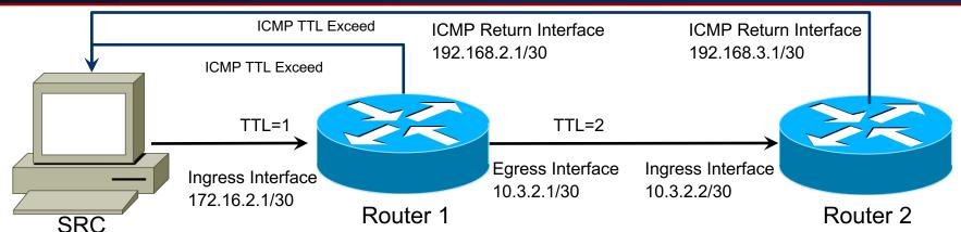
• Probe packet enters Router 1, TTL hits 0, packet is dropped
