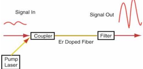
of light in the C-band spectrum, amplifying the signal.
