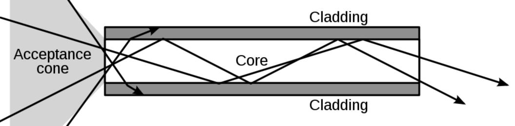
• When the light tries to pass from the core to the cladding, and the angle is correct, it is reflected back into the core.
